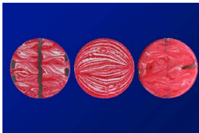
Cut views of epoxy resin mixtures produced under comparable conditions. The section on the left is of a CSE-X/8 mixture after L/D = 3. The middle section was obtained using a helical mixer after six mixing elements (L/D = 9.6). The section on the right shows a CSE-XC/4 mixture after L/D = 4.
