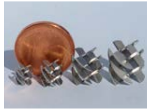
Mixing elements D_e = 4.6 to 10 mm
