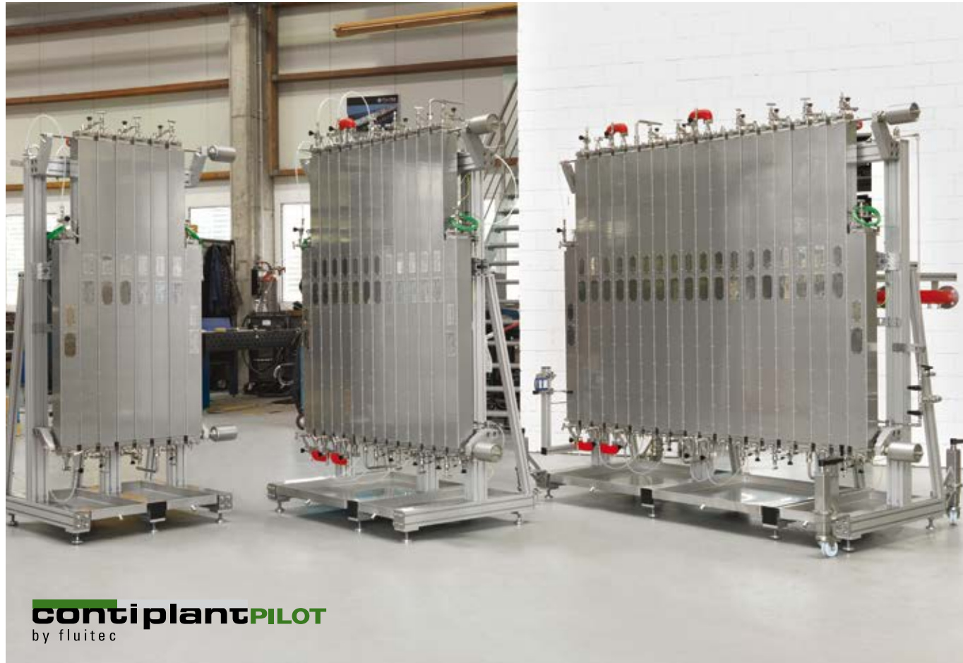
ContiplantPILOT reaction system made from Hastelloy C-22, including sampling valves, bursting discs and pressure and temperature sensors
