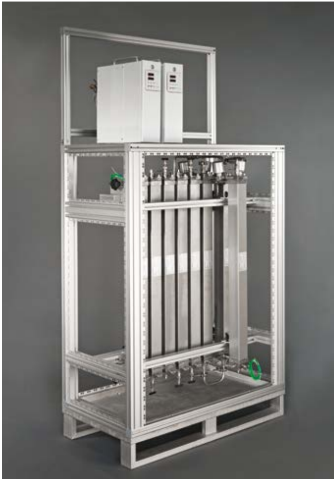
ContiplantPILOT rack with redundant reactors and residence time section
