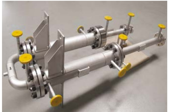
Pilot-scale polymer plant
