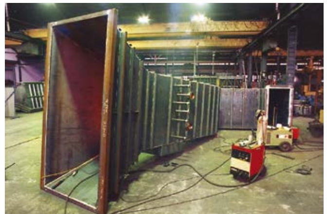
Flue gas duct for a DeNOx system
