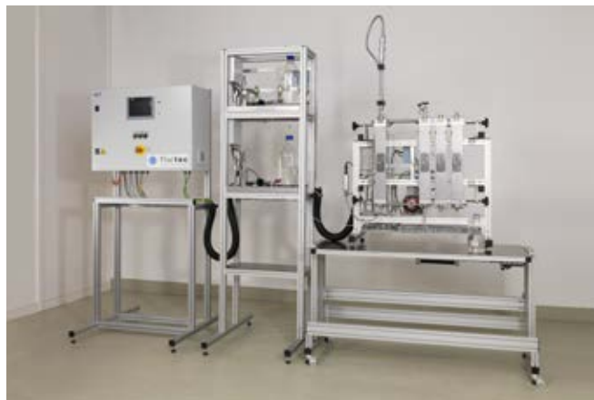
Complete ContiplantPILOT System (loop reactor with residence time section) incl. two dosing systems and PLC
