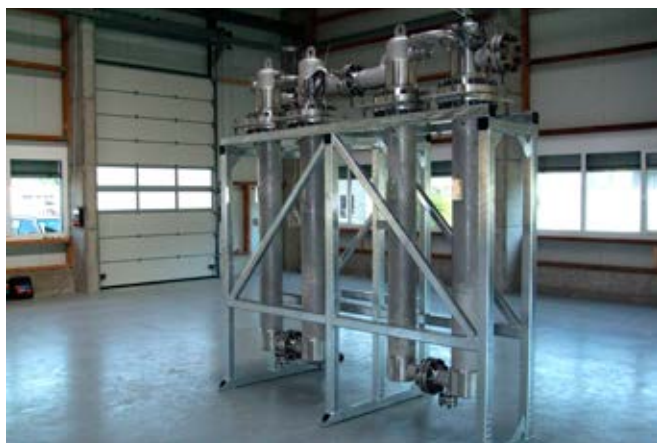
Residence time reaction section comprised of 6 Fluitec mixer / heat exchangers in line
