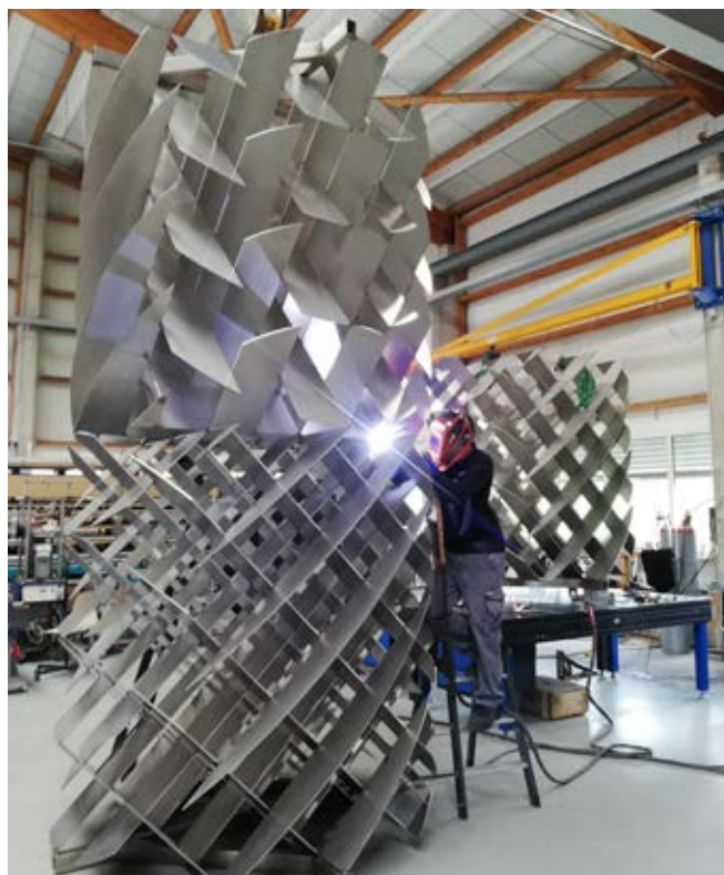
A production-scale residence time section is built
