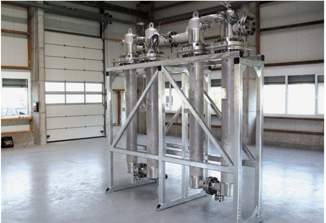
Reaction system scaled up to 4000 kg h -1
