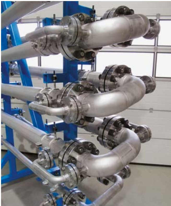
PFR reactor with 1000 kg h -1 and 20 min residence time
